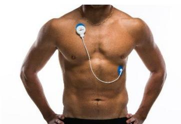
Bodyguard 2 is a lightweight device for measuring 24h HRV (RR-intervals) and 3-axis acceleration. The device is designed for robust and reliable real-life (ambulatory) measurements. The device is attached to a person using two standard electrodes and data is loaded to a PC through USB.
